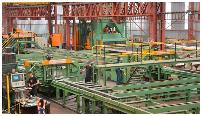
Blast machine with cross conveyor
