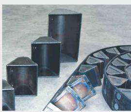
Bucket elevator belts, buckets and screws for all brands of shot blast machines
