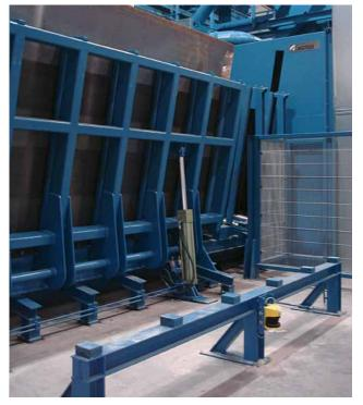
Vertical roller conveyor shot blast machine
