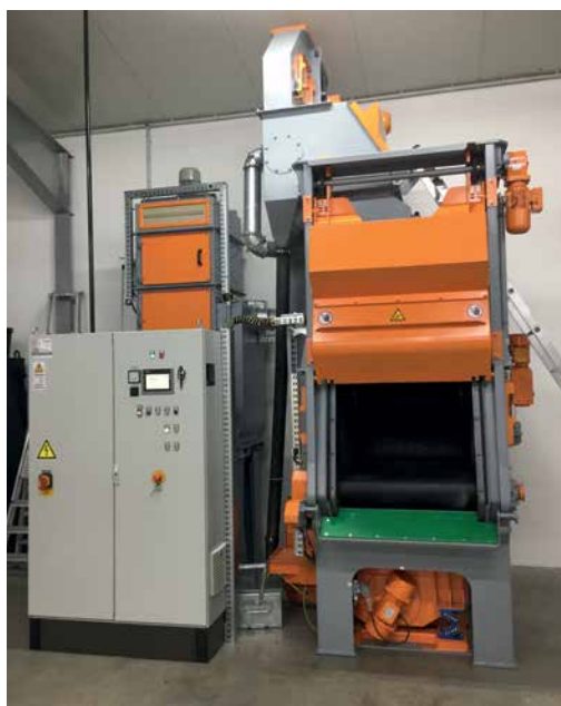
Stand-alone solution with filter unit and control cabinet
