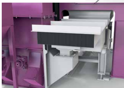
Abrasive reclamation by means of a vibro chute for immediate removal of burrs and waste parts
