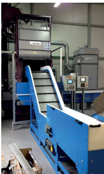
Rubber belt tumble blast machine with special loading device
