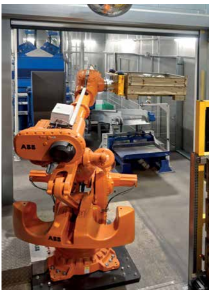
The robot is the key element of the blasting cell.
