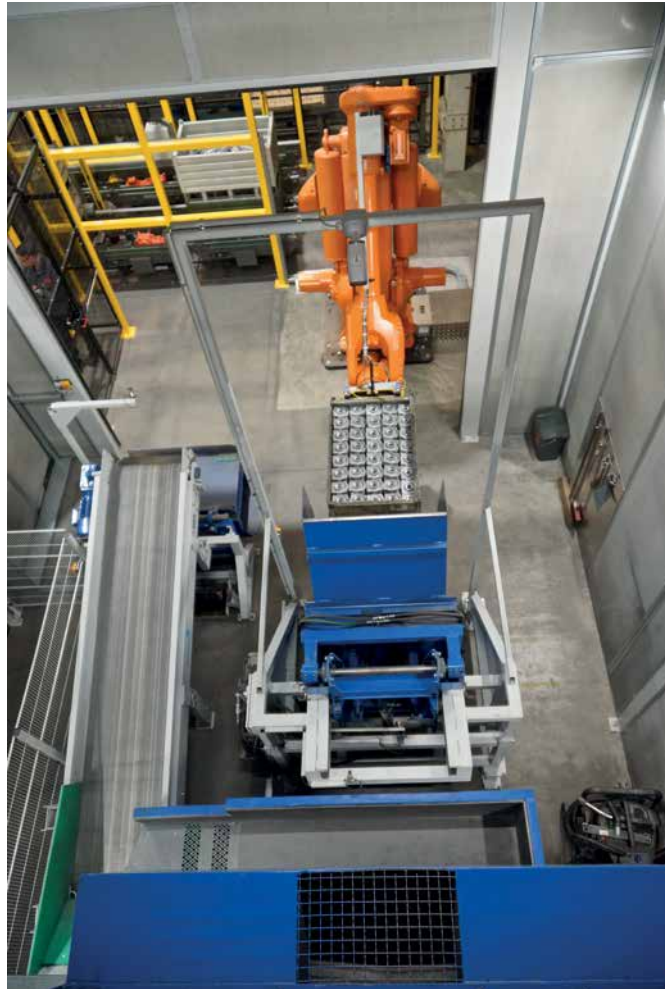
Loading the feeder of an AGTOS rubber tumble belt blast machine by means of a robot
