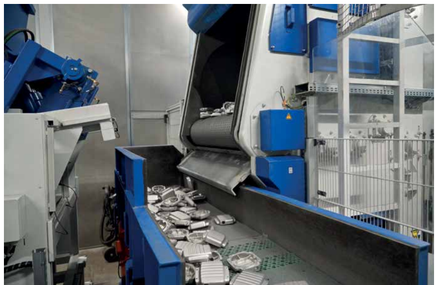
Unloading of the shot blast plant and returning the work pieces into the provided box
