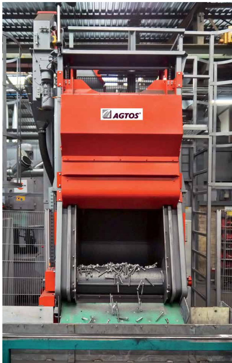
Unloading of the work pieces onto a conveyor belt and transfer to the next process step
