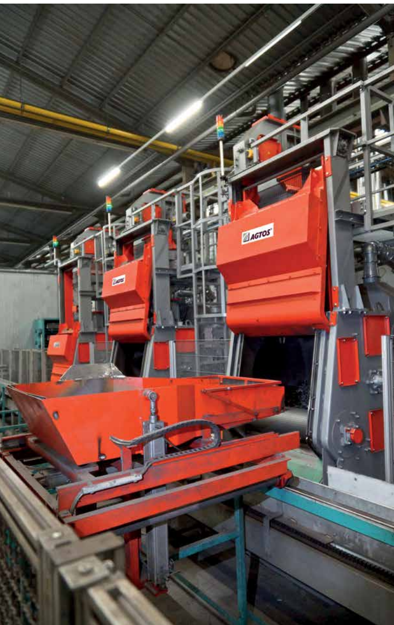
Careful loading of shot blast machines by means of loading device
