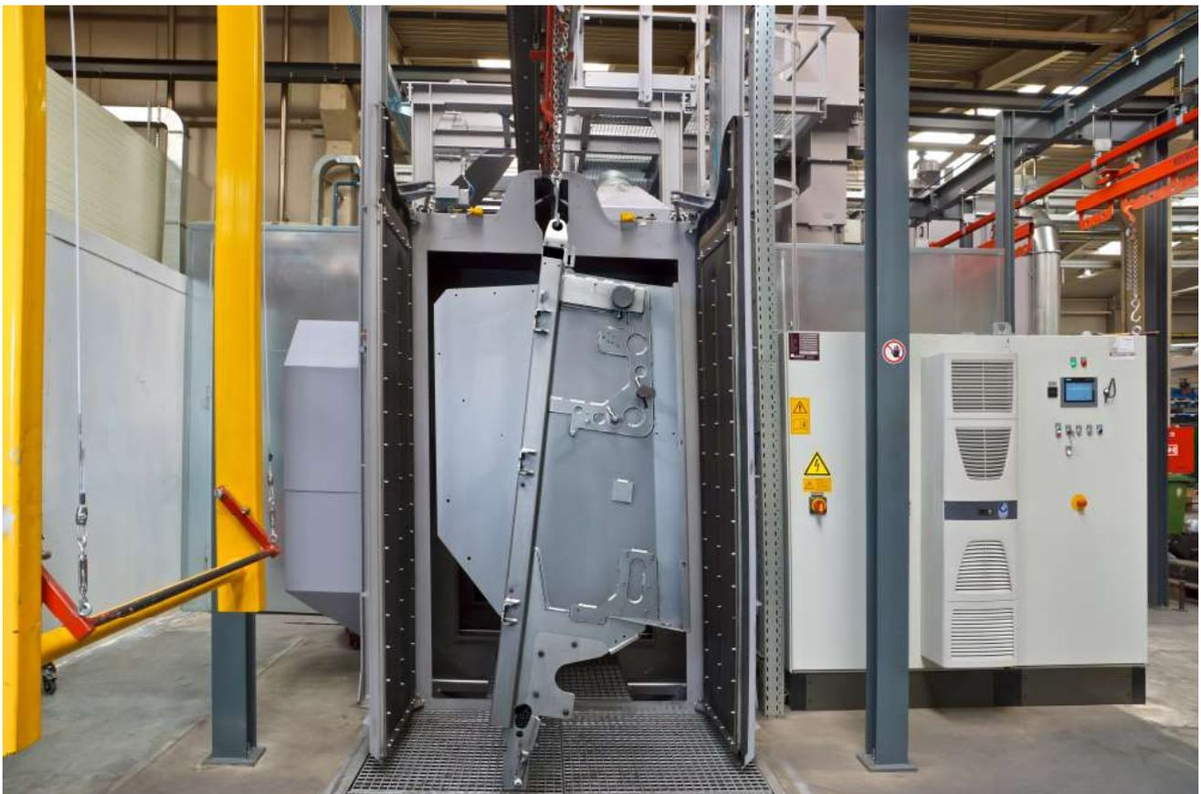
AGTOS HT 10-20-3.6-08-07.5 hanger-type shot blast machine with a blasted workpiece
