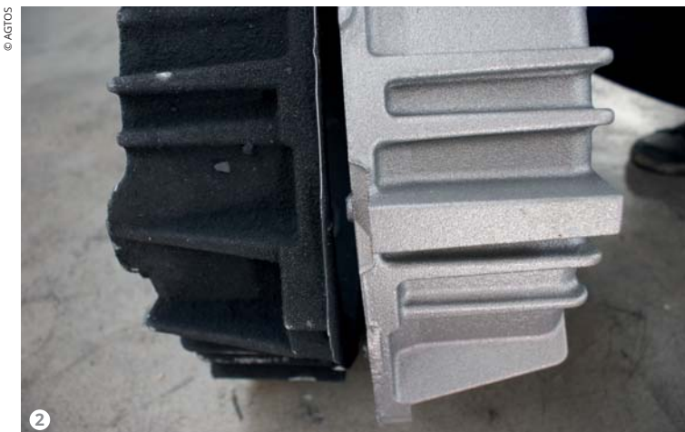
Figure 2: The blast machine by AGTOS is used for removal of sand and finishing the surfaces of casted mass products.
