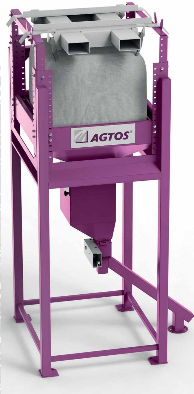
In order to ensure a continuously good blasting process, many customers are using refilling silos. The blasting media is always available in sufficient quantities and is dosed to the blasting process.
