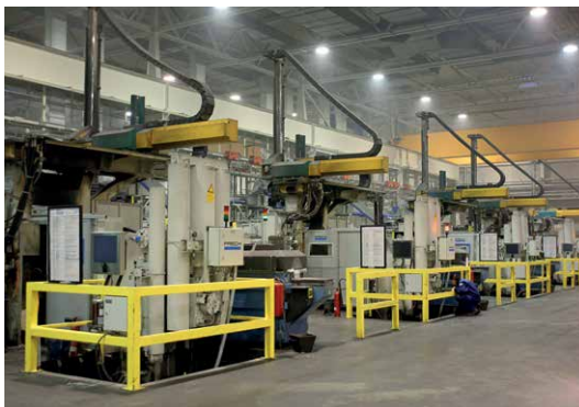
Castings which have already been deburred on the die-casting machines are fed onto a common conveyor route at half the height of the facility where they are forwarded to fine blanking.
