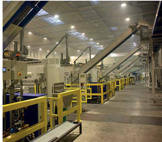
Castings which have already been deburred on the die-casting machines are fed onto a common conveyor route at half the height of the facility where they are forwarded to fine blanking.
