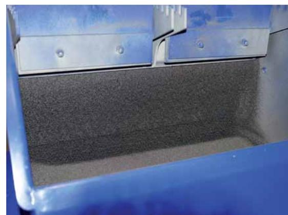
*The wind sifter eliminates dust and undersized shot from the abrasive.*
