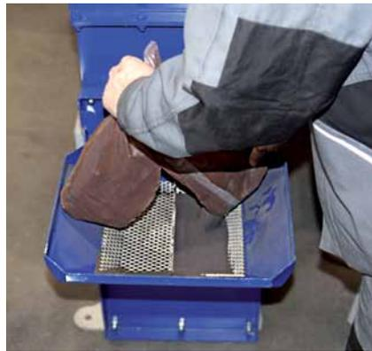
*Convenient refilling hopper for the abrasive*
