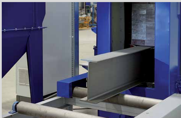
A steel girder after blasting
