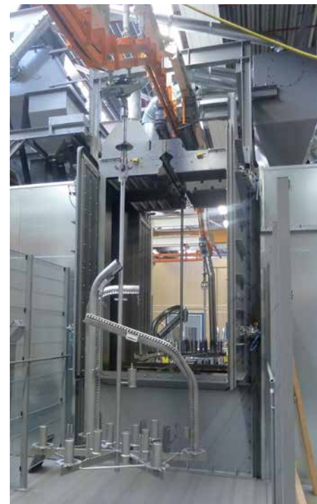
A bespoke pass-through monorail blast system for weldments
