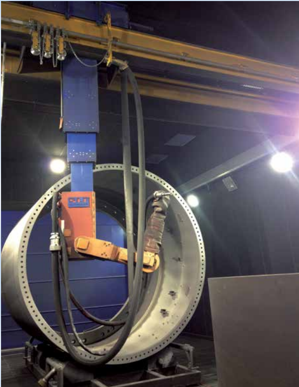
Fully automatic and highly efficient blasting of (small) series production parts with ReCo-Blast-er®
