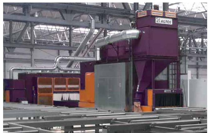
An AGTOS roller conveyor blast system with downstream paint shop and dryer
