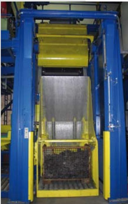
AGTOS steel mill tumble blast machine MR-850
