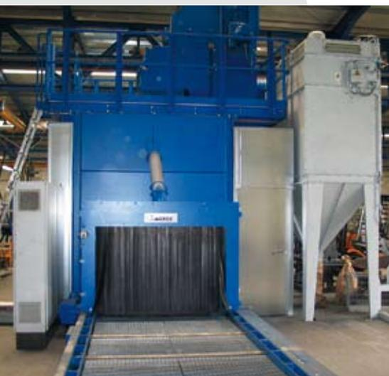
AGTOS roller conveyor blast machine RT-1500
